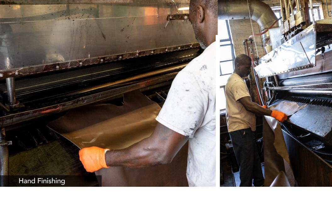
This photo shows the natural crust getting fed into a machine where it puts a little bit of dye on it, then it's hand swabbed or hand-finished.
