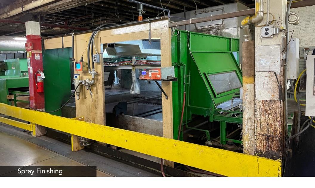
The second type of finishing done at Horween is spraying. This is where finishes are sprayed on top of the leather in a spray machine like the one you see here.
