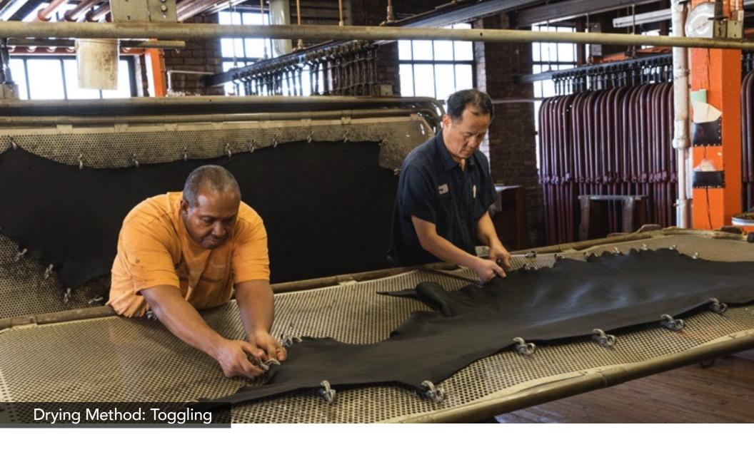
Toggling: Toggling is an older method of dying where you take clips and stretch the leather on the frame and let it air dry.
