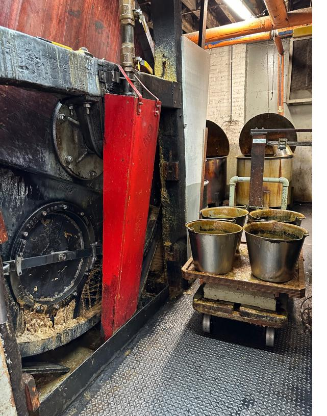
Hot stuffing Is the traditional second step in the re-tanning process for leathers that are not fat liquored or wet stuffed.
