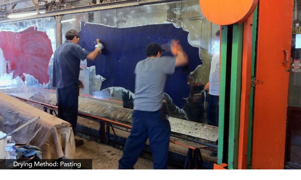
Pasting: Pasting uses a paste mixture to put the leather on a glass frame and move it through a 5-stage heater. The heater introduces heat to the leather and 4-to-6 hours after it comes out of the other pasting unit it's dry.
