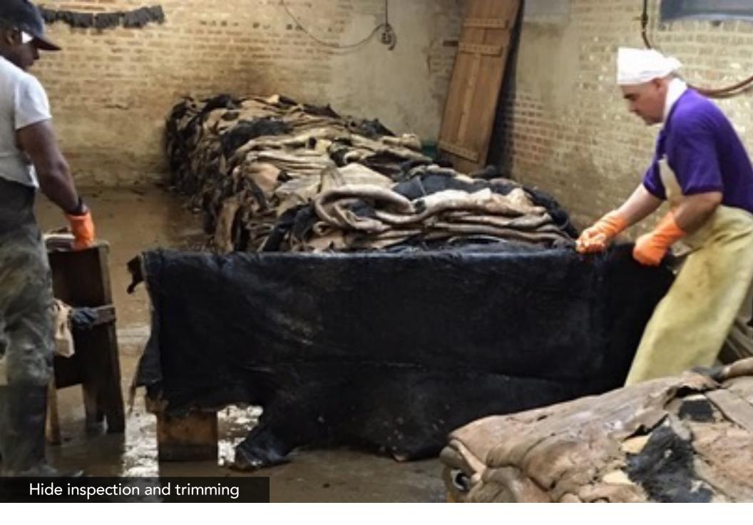
It all starts with a raw hide. What you see here is our inspection process and the trimming of hides. Once the hide is received, it's inspected for quality and the hide is processed from here.
