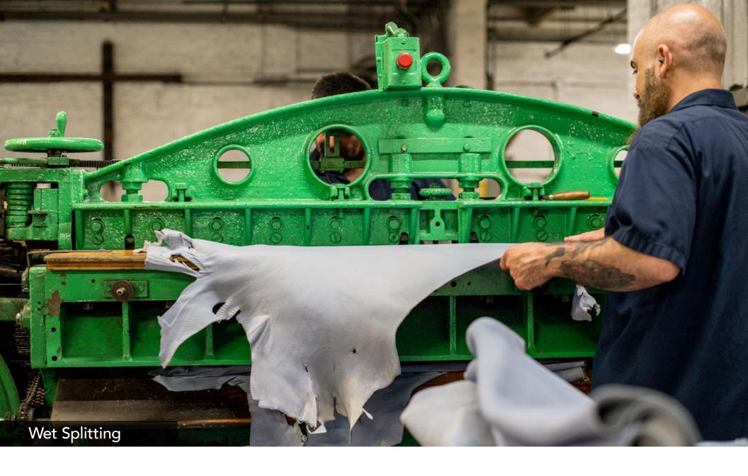
The wet blue sides are then split to the weight of the customer specifications.
