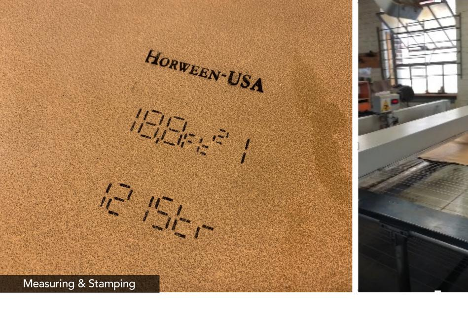
At the end of the process, we sort the leather and put a measurement on the backside of every skin.
