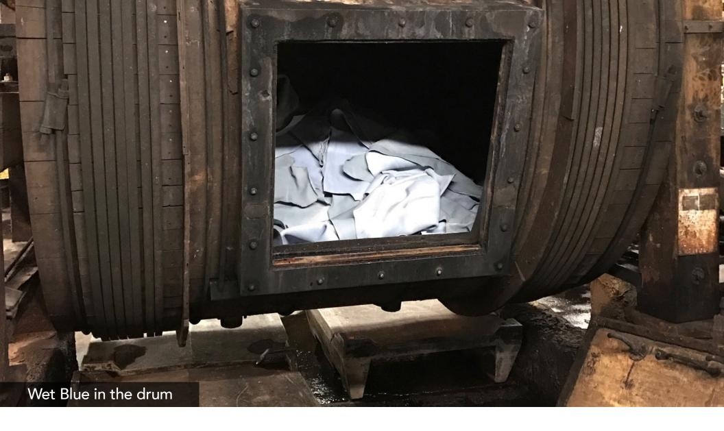
After the leather has been sorted, it's put back into a coloring drum (also called a re-tan drum).
