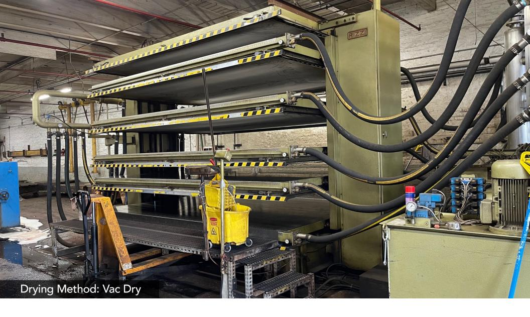
Vacuum Dry: Vacuum drying is the newest and most modern way to dry leather. Vacuum drying sucks the moisture from the leather at low heat, which gives the leather a smooth surface.
