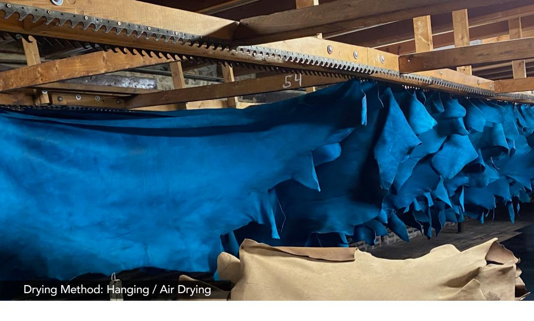
Air Drying: Air drying is a natural way to let the leather relax back into itself. The leather is put on hooks anywhere from 2 days to 10 days. Air drying lets the fibers gently come back together to create a really tight, consistent, uniform product. Air drying is an old school process, but creates a high quality yield because it lets the skin relax back into itself as opposed to other methods which can stretch the skin and fibers.
