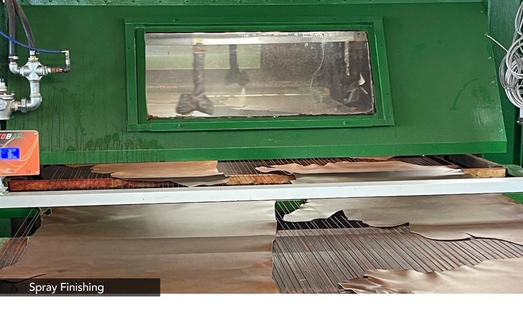
Here we have the leather being fed into the spray machine. You can see the spray guns applying the stain to the leather.
